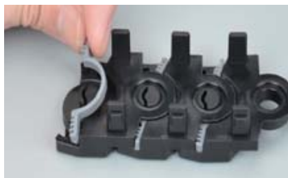
弹性元件插入侧板 Insert elastic parts into side plates
